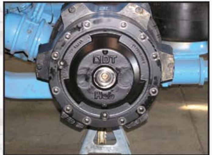
5. Cover Plate is Installed
