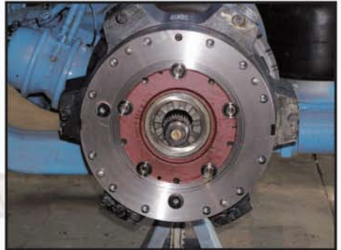
4. Axle Shaft is Installed
