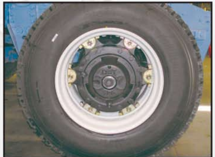
6. End plug Installed. Tires and Wheels Installed
