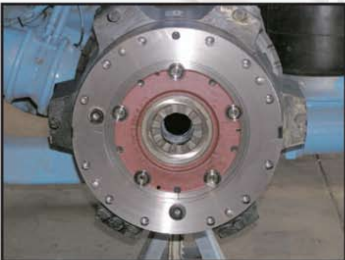
3. Planetary Gears Installed in Hub
