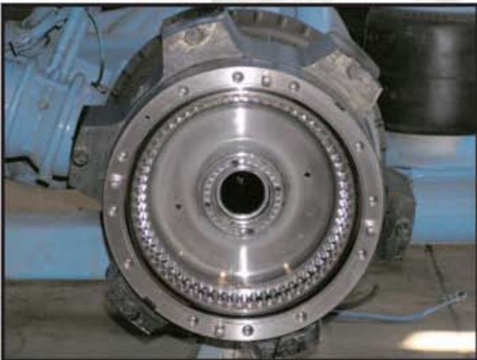
2. Hub and Ring Gear Mounted on Spindle
